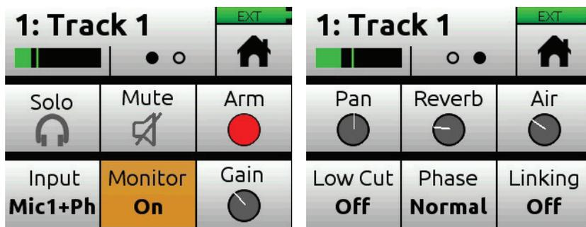
(B) Tap Input and use the HP encoder to select a source for the track. Options include: Mic, Line, Aux In, and USB In.
