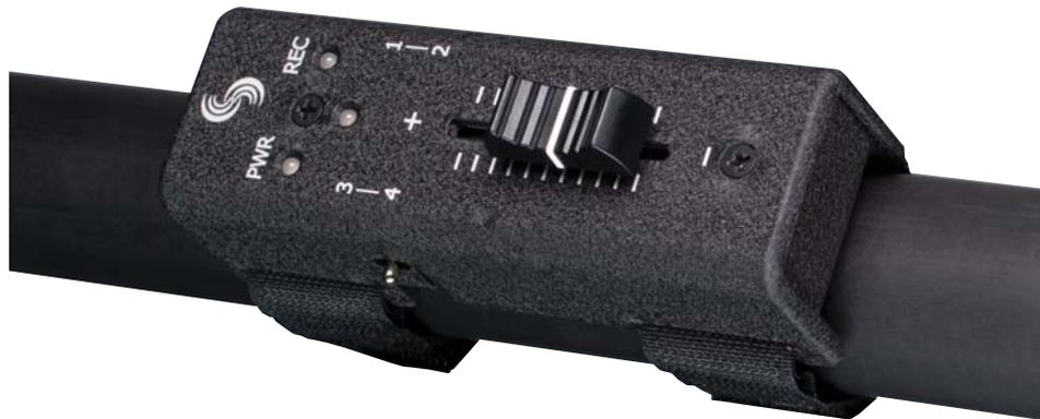
The CL-2 Remote Fader is an optional accessory for the 788T/788T-SSD Digital Recorders. The unit's linear fader can be programmed for fader control of any 788T input. The CL-2 can be mounted directly to most boom poles for easy level control of the assigned channel. The CL-2 is also usable in-hand or placed a flat surface.
