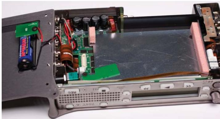
8. Place the old hard drive assembly, and the five 4-40 x 1.75" Black Oxide Phillips head screws off to the side as these are no longer needed. **DO NOT DISCARD THE TWO SMALL BLACK OXIDE PHILLIPS HEAD SCREWS.**
