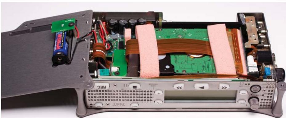
4. Loosen the screw of the small green circuit board holding down the hard drive ribbon cable.
