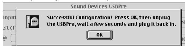
Click OK, unplug the USBPre, wait a few seconds, and reconnect. Verify the new sample rate in the USBPre control panel.
