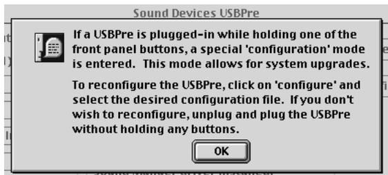
After hitting OK the USBPre control panel will open again with the Configure button available.
