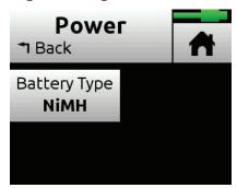
3. Select the type of batteries being used in the sled. Options include: NiMH, Alkaline, L-Mount
