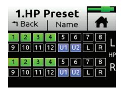
Incorrect routing of USB sources within the input or headphone matrix may cause feedback.
