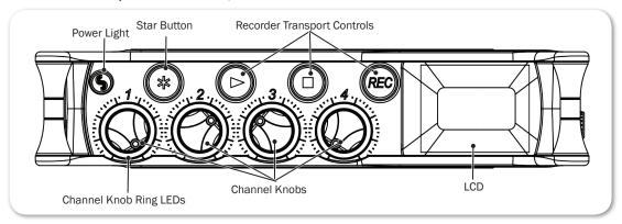
The Channel knobs on the front panel have two purposes:
