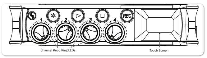
The LEDs around any of the knobs will also pulse orange if, upon changing track banks, the knob's rotational position is not aligned with its fader value; this pulsing stops once position and value are realigned. For more information, see *Track Bank Selector*.
