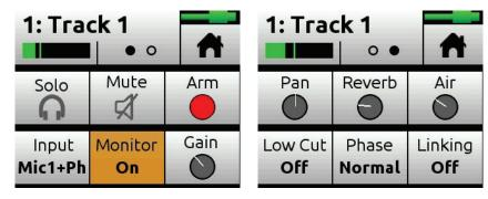
Each Channel screen provides two pages of settings—indicated by Dots icon. Tap the Dots icon to switch pages.
