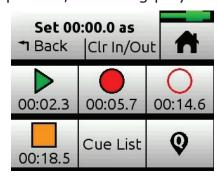
① It is not possible to place an In point after an Out point. It is also not possible to have more than one In or Out point of each type (Play or Record).
