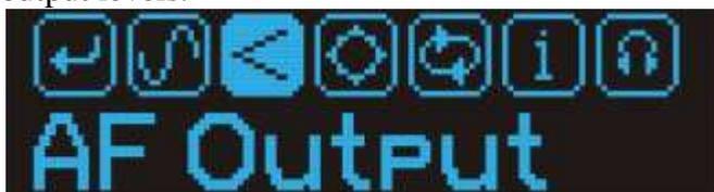
The receiver output level can be set to any one of 4 pres-set levels in 12dB steps. Scroll the nav-switch left or right to select the desired value is . Press and hold the nav-switch to confirm the choice of output level.
