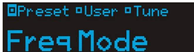
In **Tune** mode the user can select any frequency within the switching bandwidth of the frequency table in 25kHz steps and then save them to the **User** memory. The User memory is initially programmed with a copy of the **Preset** frequencies until the user selects and saves a frequency in **Tune** mode.
