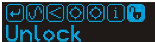
To unlock the transmitter, scroll to the unlock symbol and use the middle part of the navigation switch to select the Yes option. The transmitter will then return to the main menu.
