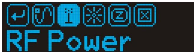
In selecting the RF Power from the Options menu the user can select High or Low power settings. In selecting the low power setting the user will extend the battery life of the transmitter.
