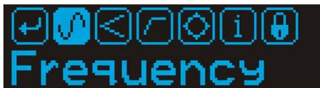
After accessing the main menu, use the navigation switch to scroll to the Frequency option. Once the frequency option is highlighted, press down on the nav switch to enter the frequency menu to view the range of frequencies.
