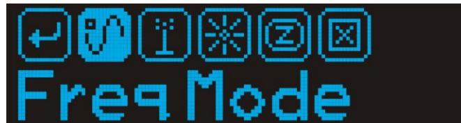
In selecting the frequency mode the user can select one of three frequency modes, Factory set **Preset**, **User**, or manual **Tune**.
