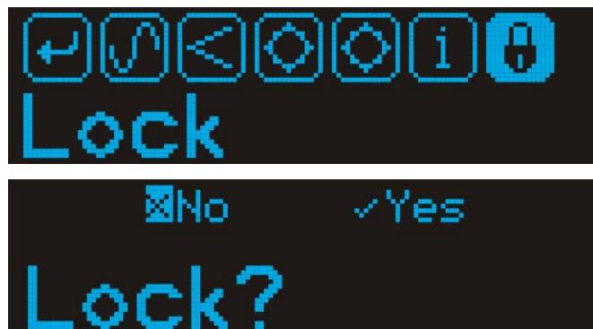
To lock the transmitter, scroll using the navigation switch to the Yes option. The transmitter will then return to the main menu, with an unlock symbol to replace the lock symbol.
