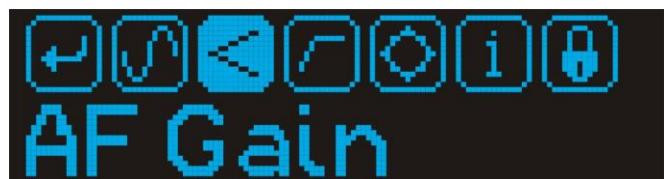
After accessing the main menu, use the navigation switch to scroll to the AF gain option. Once the AF gain option is highlighted, press the nav switch to select one of 10 AF gain settings.
