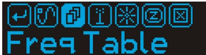
Units which are programmed with multiple tables will show frequency table selection on the menu. Entering the frequency table selection screen will show the frequency table number. The user can select any one of up to 10 tables.
