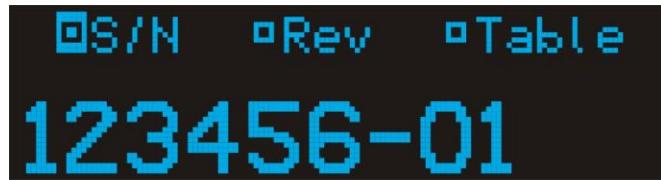
To view the information for any of these, there is no need to press down the middle button. Simply scrolling from left to right will enable you to view the data for any of the three headings. Pressing down on the navigation switch will instantly take the transmitter back to the Main Menu.
