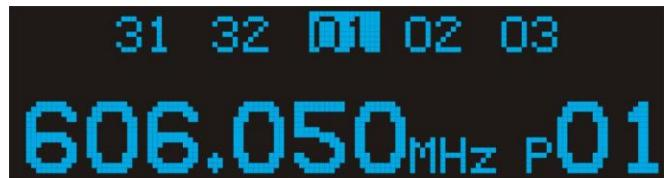
A range of frequencies will be displayed and the desired one can be highlighted using the scroll. To confirm the desired frequency press down on the navigation switch to make the selection. The transmitter will then return to the main menu.
