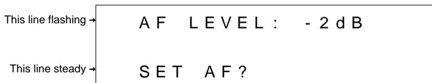
Fig:8 AF ATTENUATOR SETTING SCREEN.
