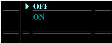
The currently programmed mast-head supply state is indicated by the flashing arrow-head cursor to the left of the option text.
