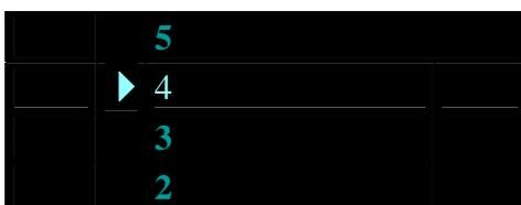
The flashing arrow-head cursor indicates the current brightness setting. Move it up or down to the required brightness level, then press the **OK** button.
