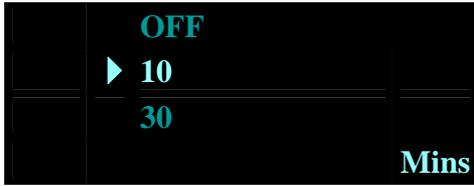
If the OFF setting is selected, the screen saver feature is disabled, otherwise, it shuts down the OLED display when no buttons have been pressed for the selected time (10 minutes or 30 minutes).
