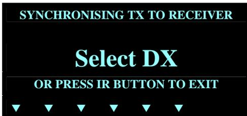
A flashing 'down-arrow' cursor will be displayed above the receiver selection button for each receiver that the RK6 rack was able to interrogate via the IrDA interface.
