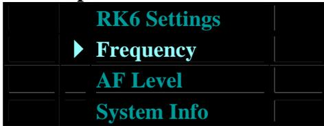
The currently indexed option is indicated by the flashing arrow-head cursor to the left of the option text.
