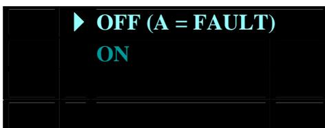
The top line will show 'OFF (A = FAULT)' or 'OFF (B = FAULT)', depending on which amplifier tripped the power supply.
