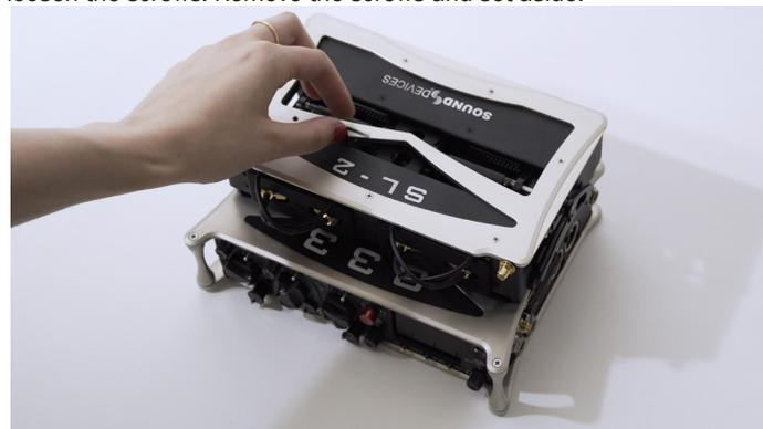
**STEP 5** Replace the originally provided rear black screws near the Sound Devices logo using #4 Phillips head screwdriver.
