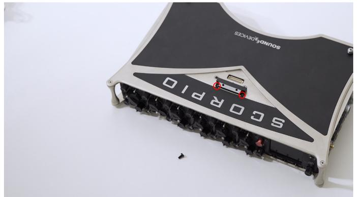
**STEP 5** If desired, remove the additional Scorpio mounting hardware from the SL-2.
