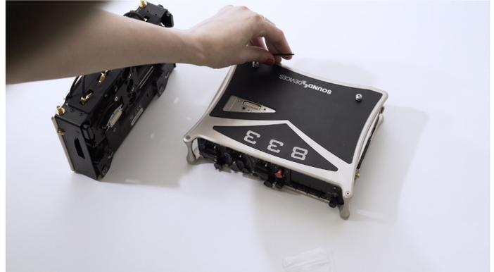
**STEP 4** Align the SL-2's bottom panel hooks with the Rear Keyhole Pegs on the 833/888. The SL-2 should be tilted with the front panel slightly higher than the rear. Take care not to bump the SL-2 expansion connector against the 833/888 top panel. Once the SL-2's Bottom Panel hooks and Rear Keyhole Peg's machined grooves are aligned, slide the SL-2 towards the front panel.
