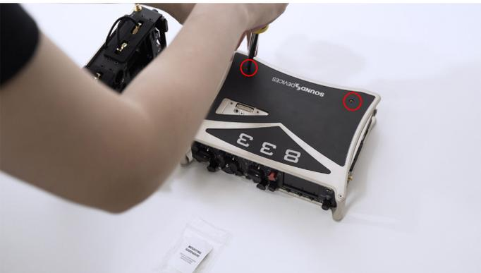
**STEP 3** Using the provided 2 mm Allen Wrench, screw in two Rear Keyhole Pegs into the threads where you removed the screws in Step 2.
