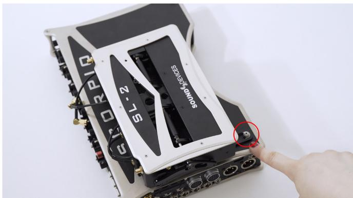
**STEP 3** Remove the two small black screws.
