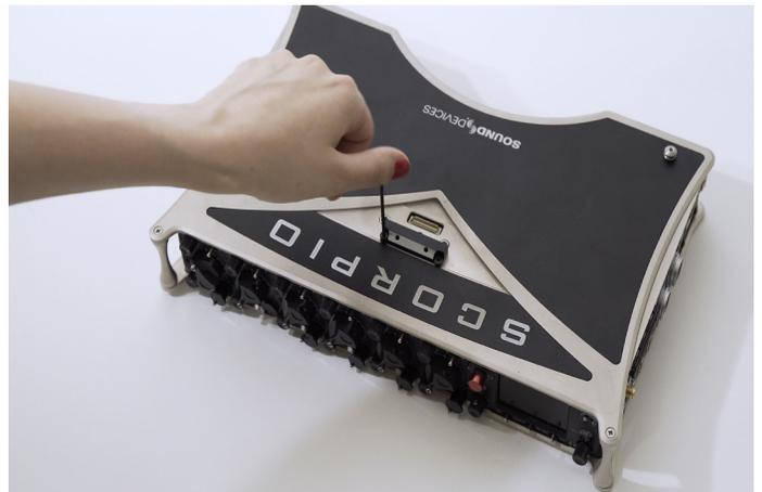
**STEP 4** Remove the safety mount from the top panel of Scorpio.
