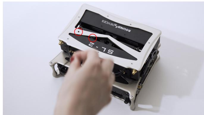
**STEP 2** Insert the allen wrench into these holes, visually confirming that the wrench is in contact with the safety screws inside the SL-2. Turn the wrench counterclockwise to loosen the screws. Remove the screws and set aside.
