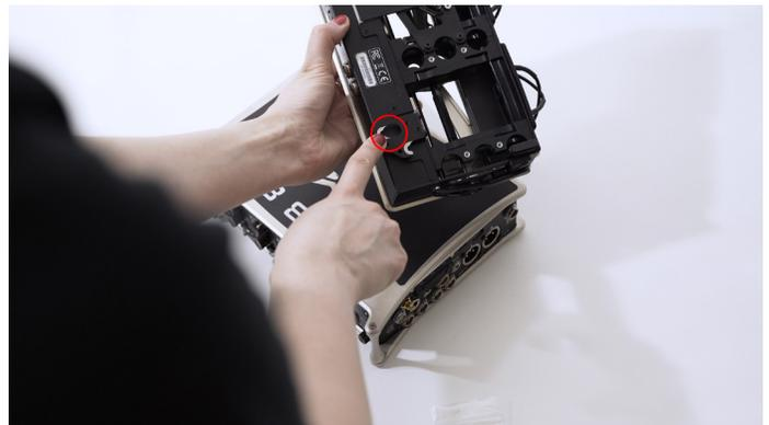
**STEP 5** Make sure that the SL-2 Expansion Connector mates with the 833/888 Expansion Port. Then gently press down on the SL-2 to fully seat the pins of the connector.
