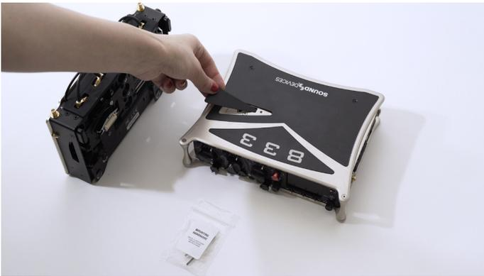
**STEP 2** Using a #4 Phillips Screwdriver, remove the two black phillips screws from the Scorpio top panel as shown in the image below. Keep these screws in a safe place as they need to be re-installed if the SL-2 is removed from the 833/888.
