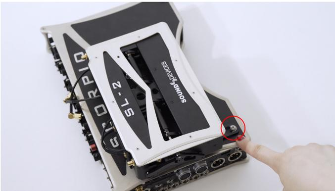
**STEP 7** Make sure that the SL-2 Expansion Connector mates with the Scorpio Expansion Port. Then gently press down on the SL-2 to fully seat the pins of the connector.
